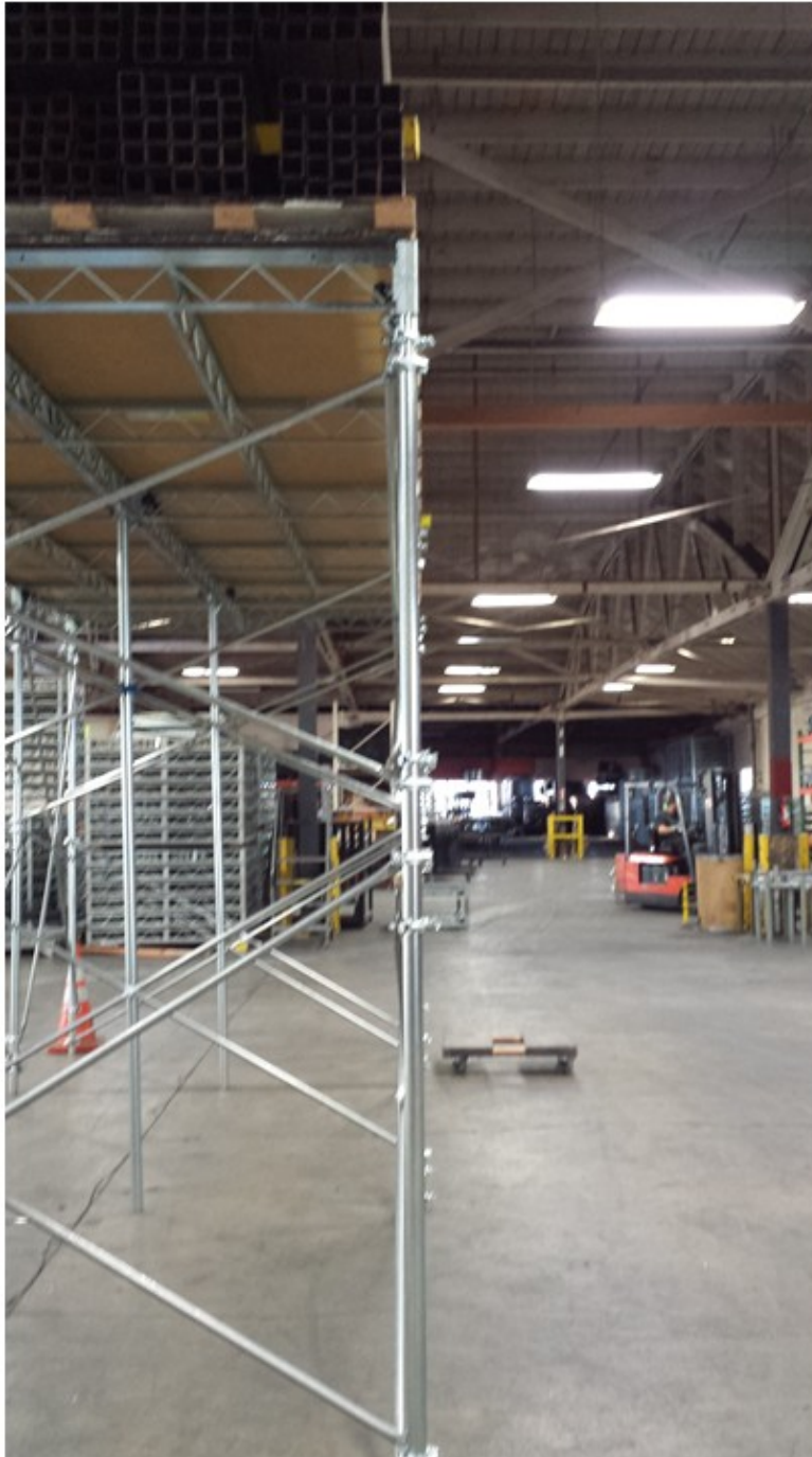
Figure 3-4 Load Step 1, Platform loaded to 202.76 lbs/ft 2
