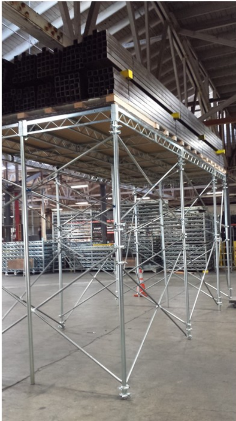
Figure 3-2 Load Step 1, Platform loaded to 202.76 lbs/ft 2
