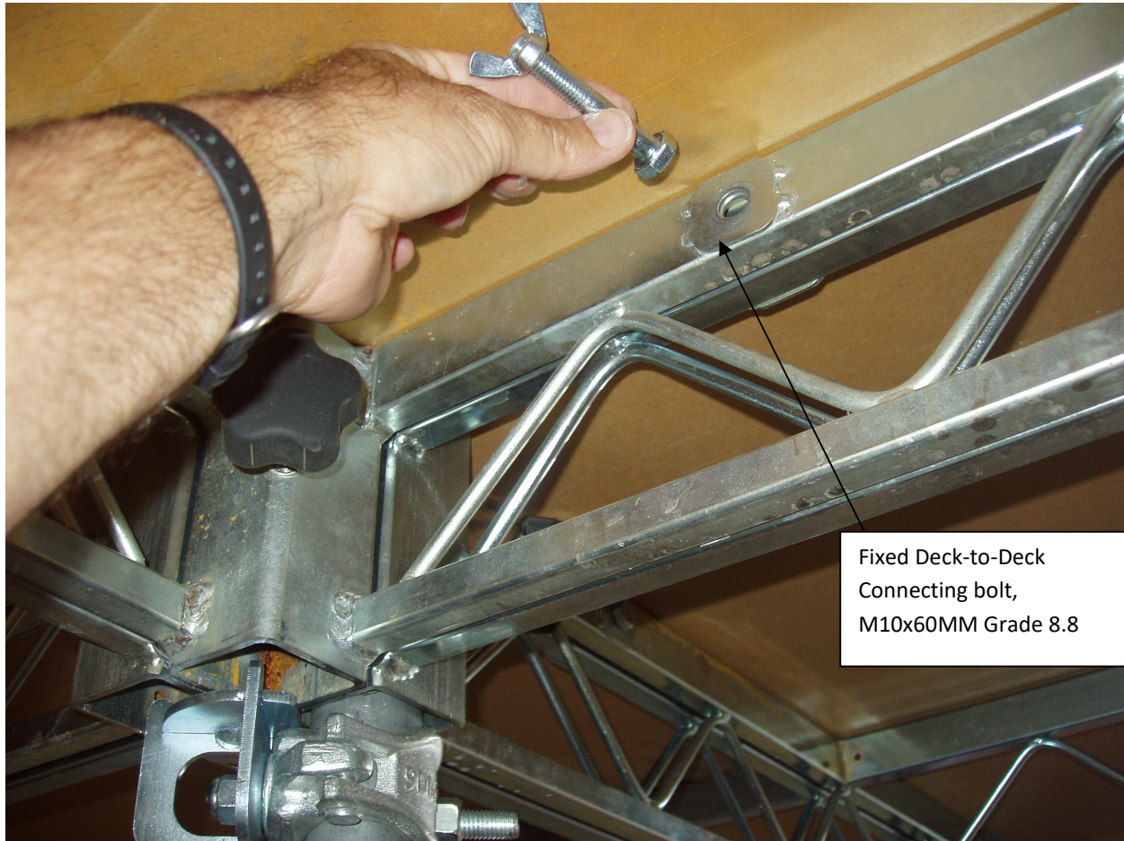
Figure 1-4 Typical STEELDECK® Deck-to-deck Connecting Bolt Joint
