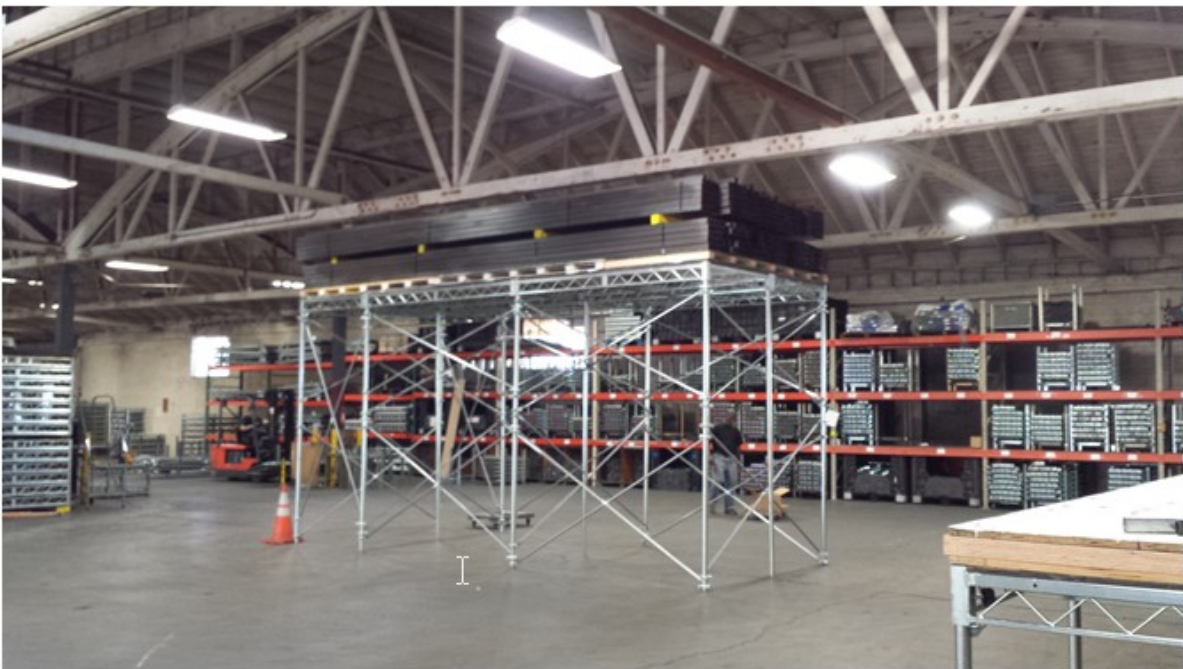
Figure 3-1 Load Step 1, Platform loaded to 202.76 lbs/ft 2
