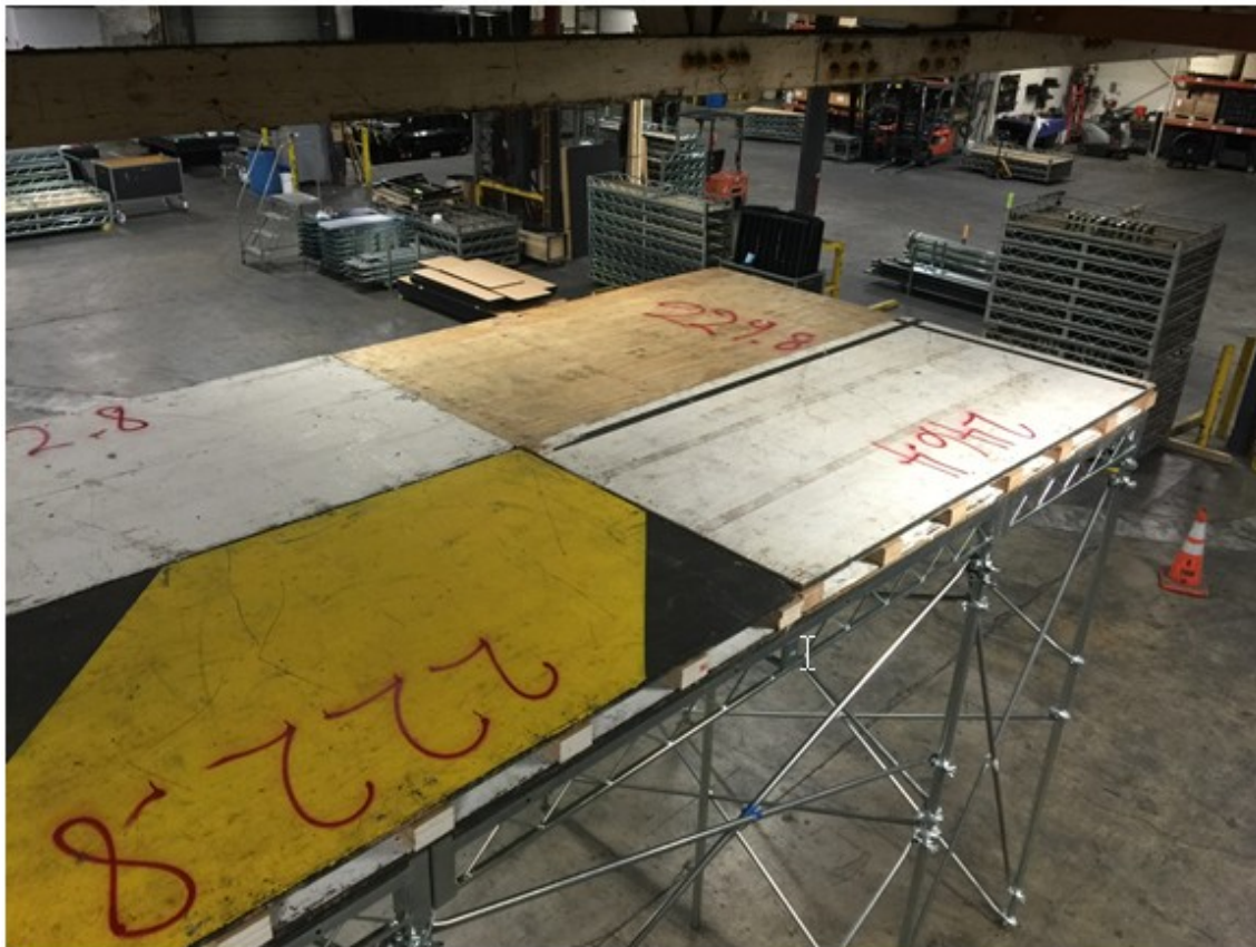
Figure 2-8 10 ft. tall 8x20 ft. Platform with \geq 221 lb wooden pallets in place, overlapping deck seams
