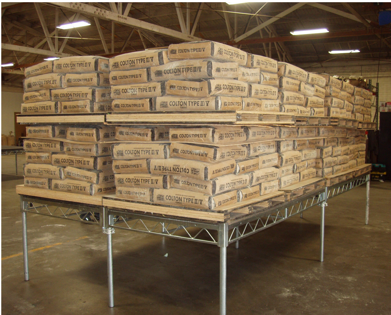
Figure 1-8 3 Ft High Platform loaded to 271.0 lbs/ft 2
