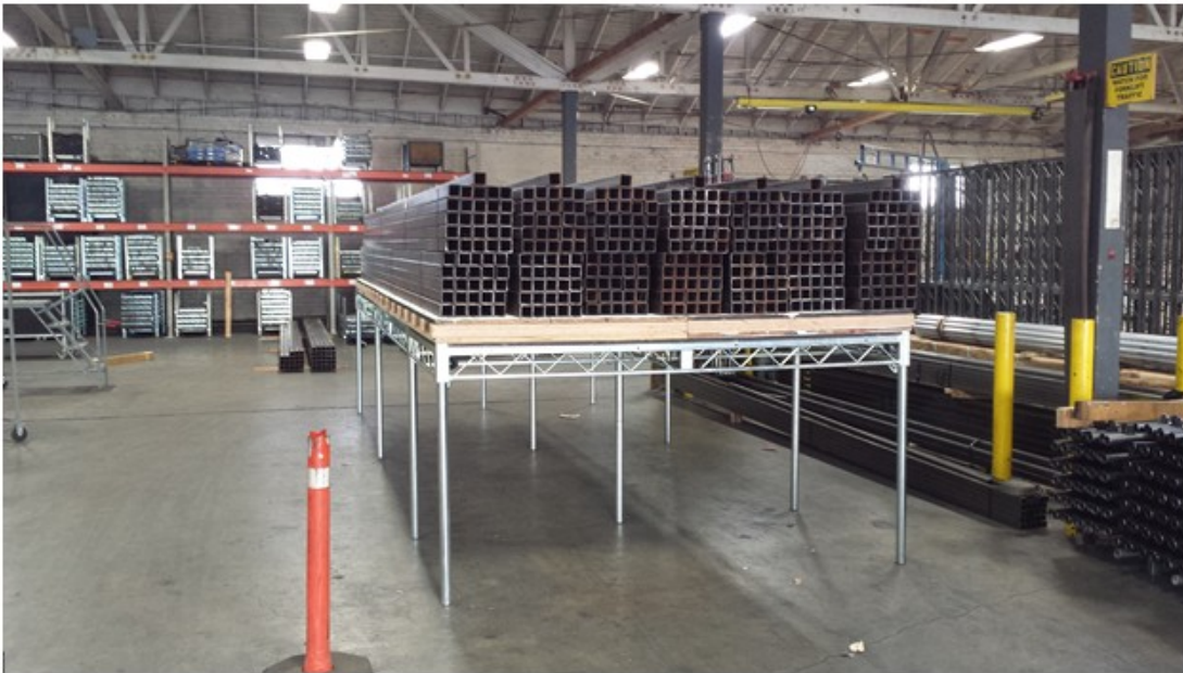
Figure 1-9 4 Foot High Platform loaded to 202.76 lbs/ft 2
