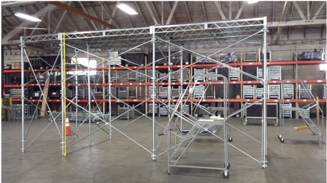
Figure 2-1 Test Platform, 10 ft high
