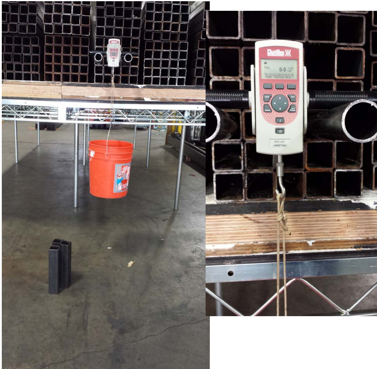
Figure 2-5 Zeroed out load cell with empty bucket
