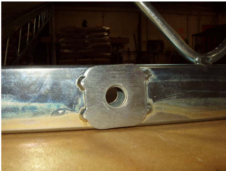
Figure 3-8 No distress of critical deck-to-deck bearing surfaces
