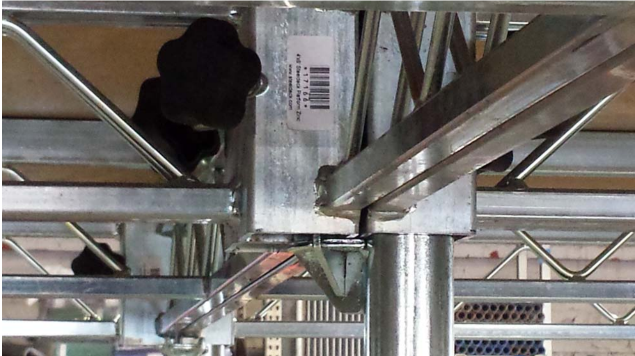
Figure 3-7 No distress of critical leg-to-deck support mount
