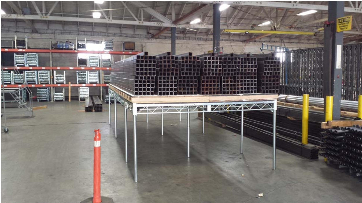
Figure 1-9 4 Foot High Platform loaded to 202.76 lbs/ft 2
