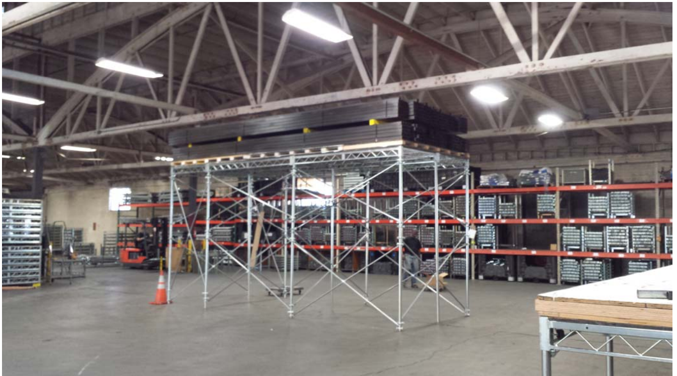
Figure 3-1 Load Step 1, Platform loaded to 202.76 lbs/ft 2
