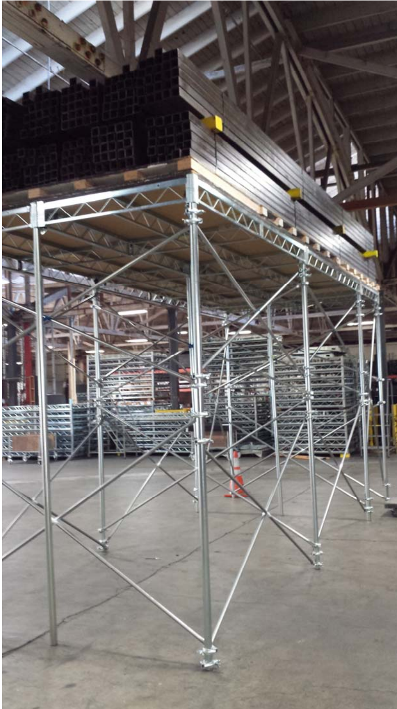
Figure 3-2 Load Step 1, Platform loaded to 202.76 lbs/ft 2
