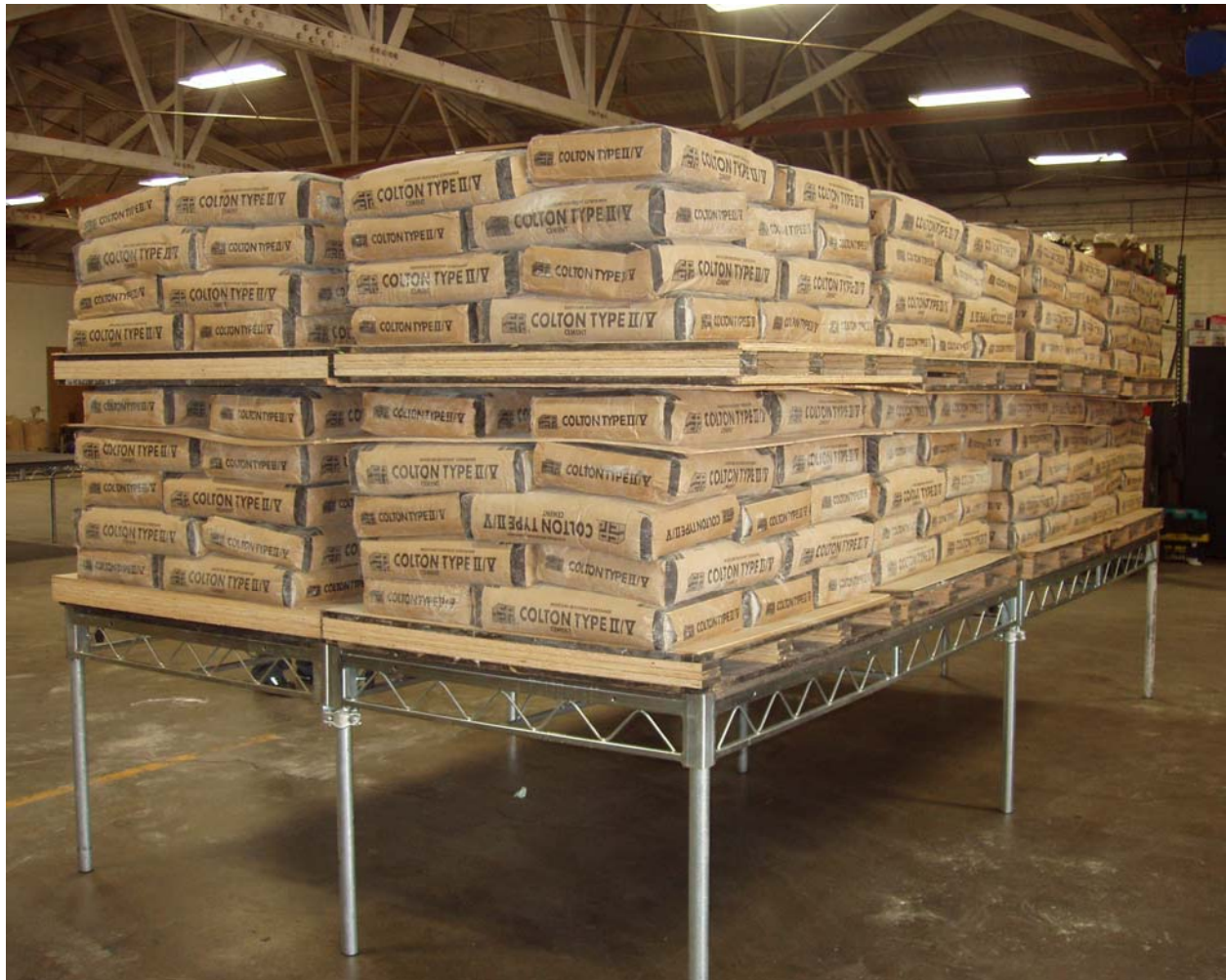
Figure 1-8 3 Ft High Platform loaded to 271.0 lbs/ft 2
