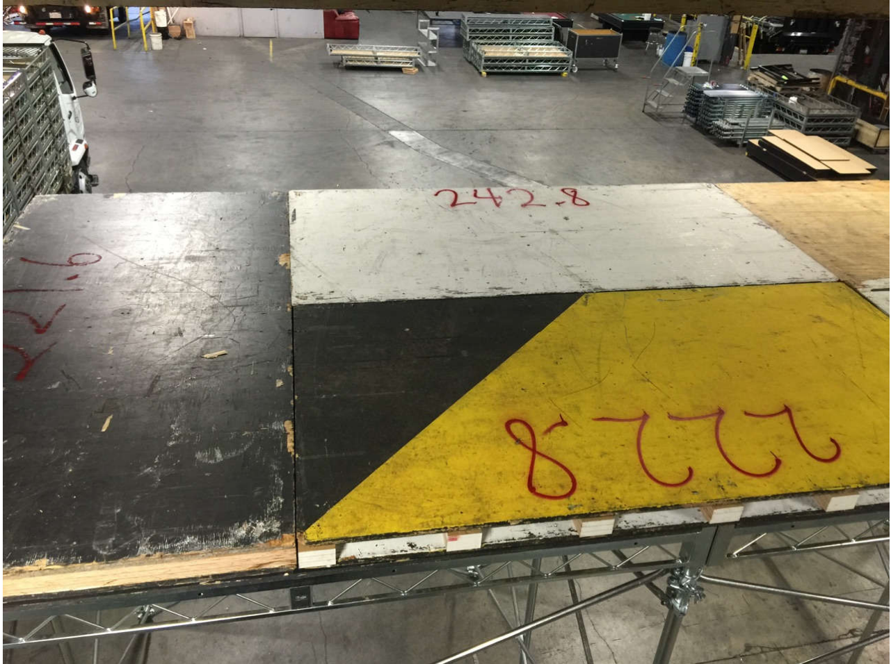
Figure 2-9 10 ft. tall 8x20 ft. Platform with \geq 221 lb wooden pallets in place, overlapping deck seams
