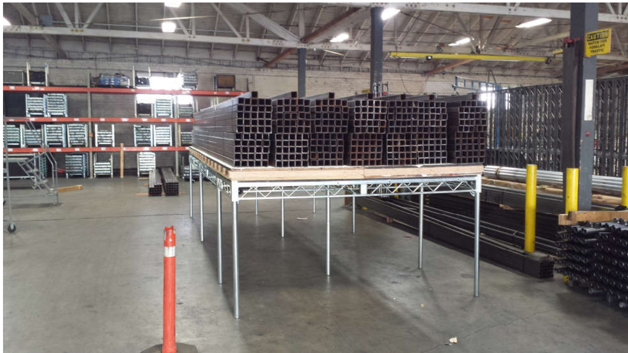
Figure 1-9 4 Foot High Platform loaded to 202.76 lbs/ft 2
