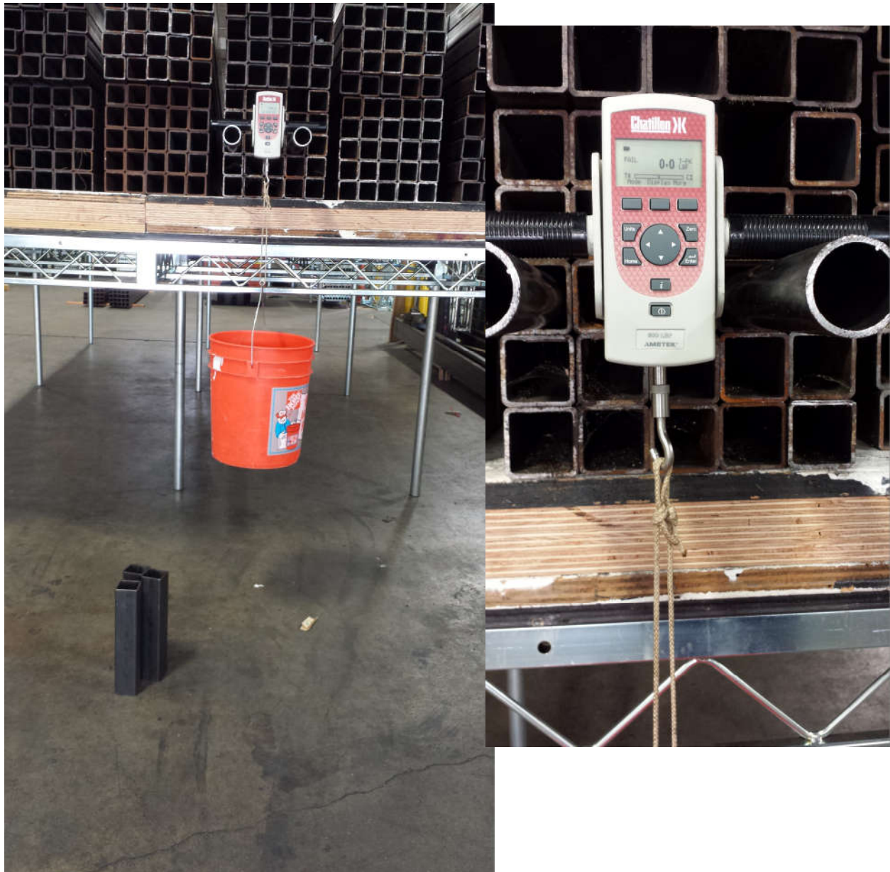
Figure 2-5 Zeroed out load cell with empty bucket
