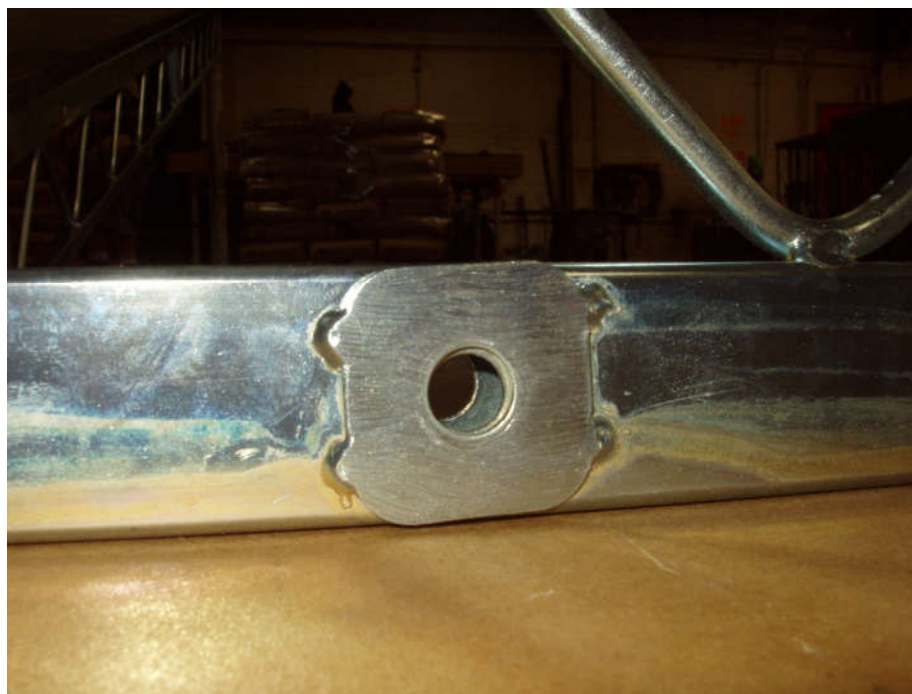
Figure 3-8 No distress of critical deck-to-deck bearing surfaces
