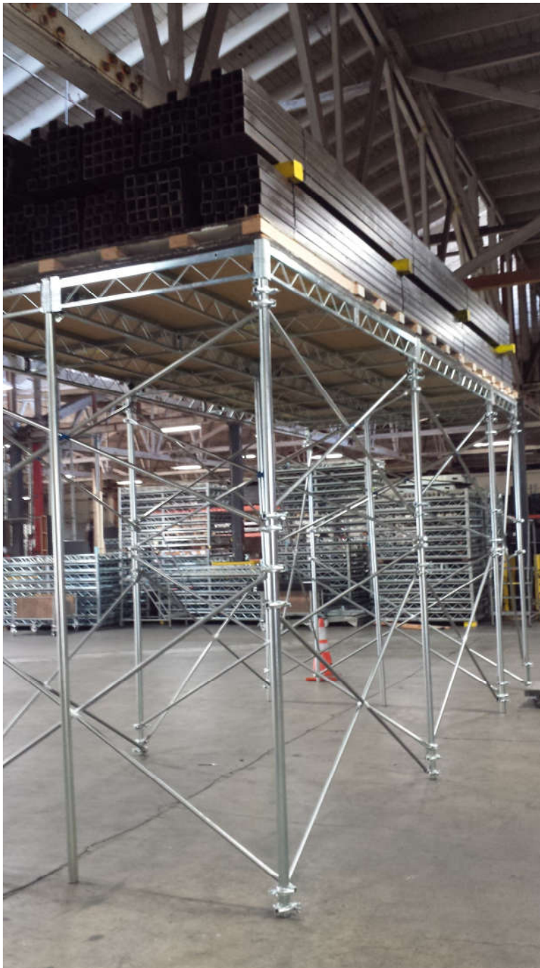
Figure 3-2 Load Step 1, Platform loaded to 202.76 lbs/ft 2
