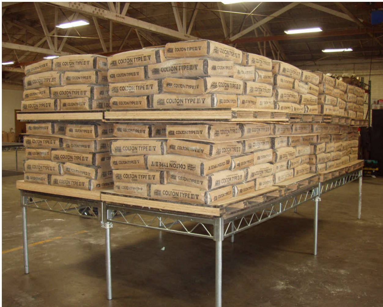
Figure 1-8 3 Ft High Platform loaded to 271.0 lbs/ft 2
