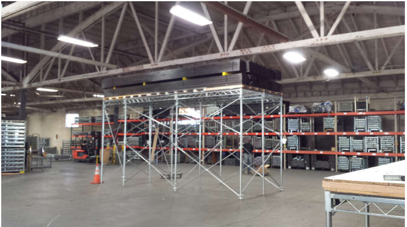
Figure 3-1 Load Step 1, Platform loaded to 202.76 lbs/ft 2
