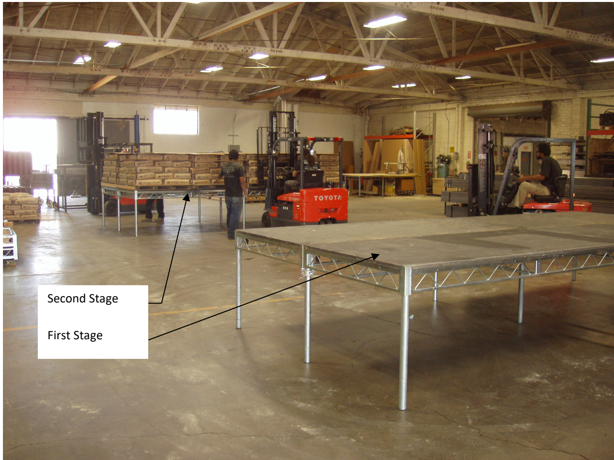
Figure 3-7 Load Step 4, 2 nd Platform loaded to 147.25 lbs/ft 2
