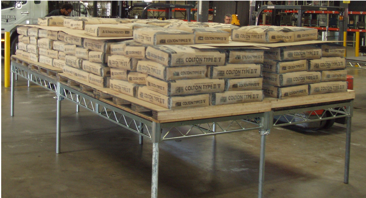
Figure 3-1 Load Step 1, 1 st Platform loaded to 135.5 lbs/ft 2
