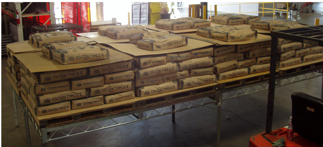
Figure 2-6 First Platform loaded to 135.5 lbs/ft 2
