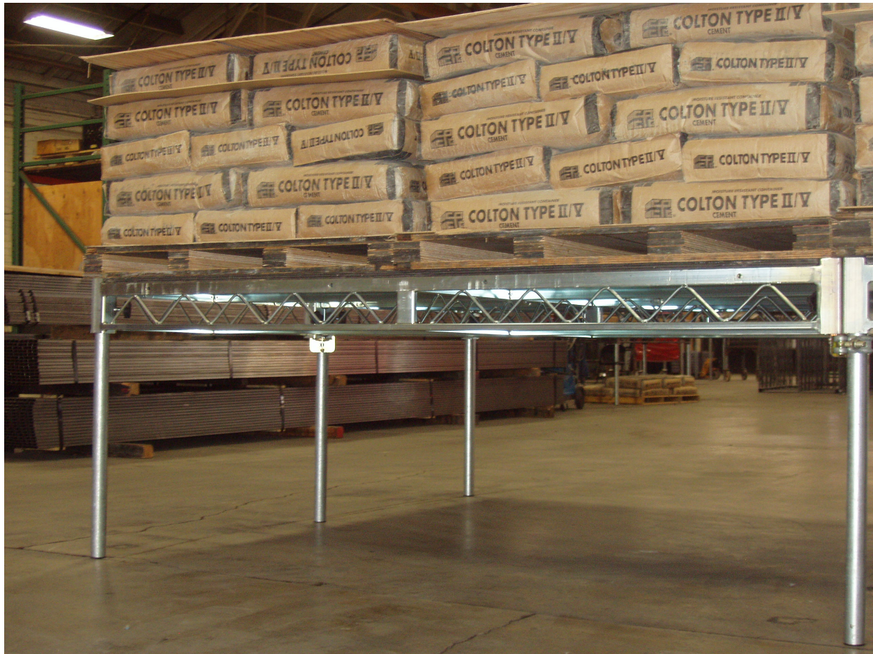
Figure 3-8 Load Step 4, 2 nd Platform loaded to 147.25 lbs/ft 2 , 3/16" Sag of 8' long beams
