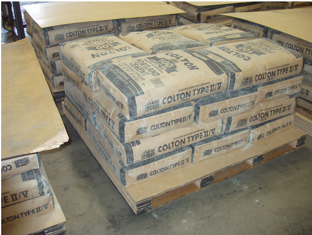
Figure 2-4 Symmetrically loaded pallet
