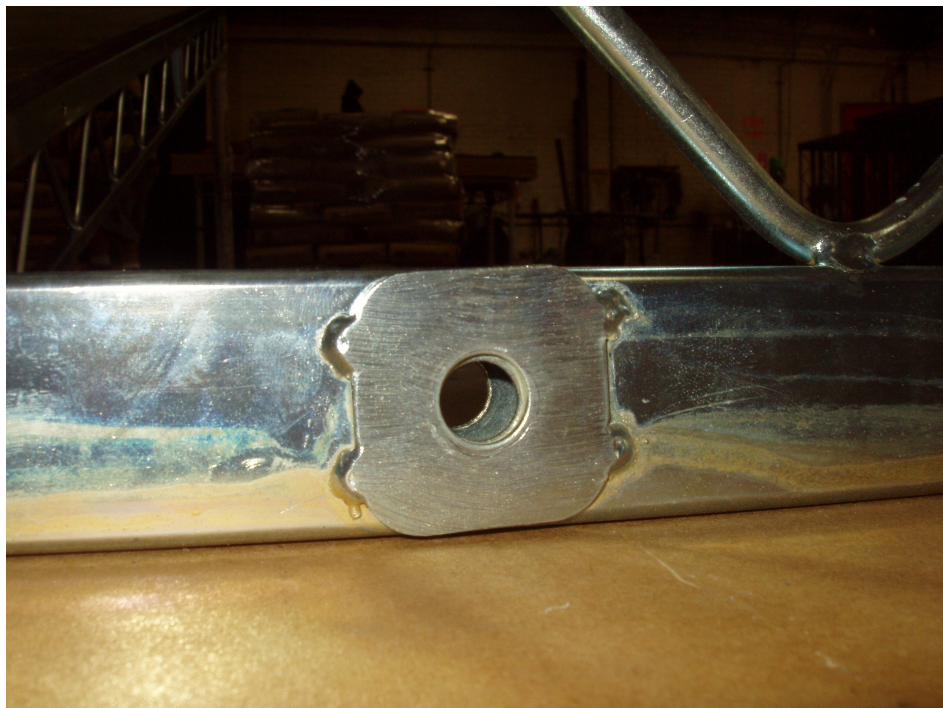
Figure 3-10 Load Step 15, 2 nd Platform, No distress of critical deck-to-deck bearing surfaces
