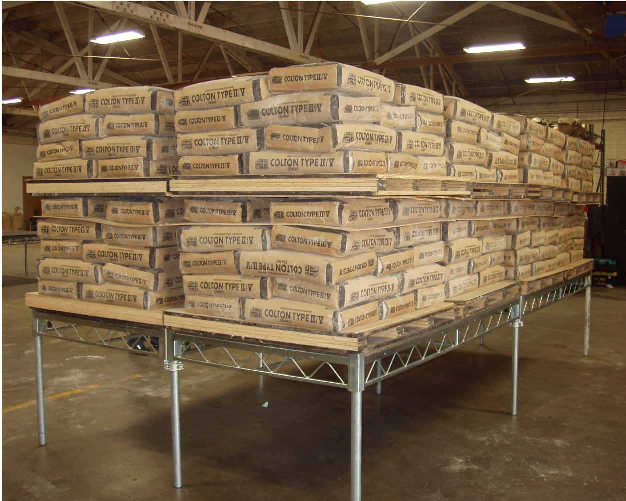
Figure 3-2 Load Step 2, 1 st Platform loaded to 271.0 lbs/ft 2
