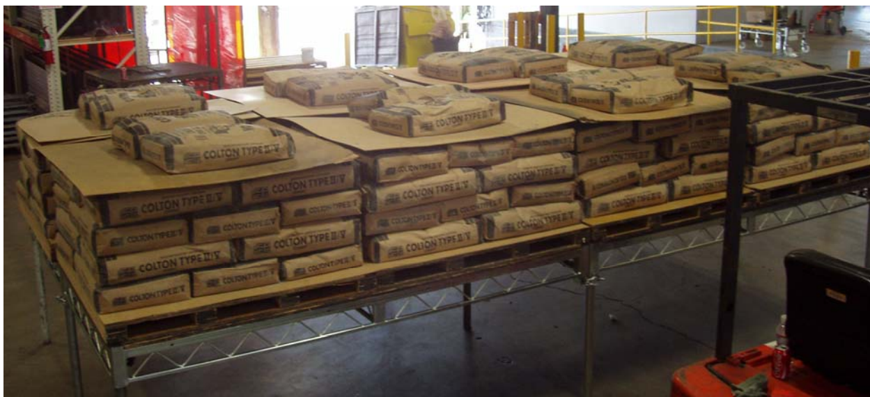
Figure 2-6 First Platform loaded to 135.5 lbs/ft 2
