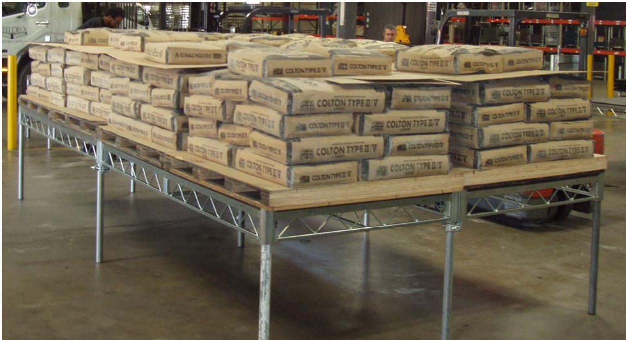
Figure 3-1 Load Step 1, 1 st Platform loaded to 135.5 lbs/ft 2
