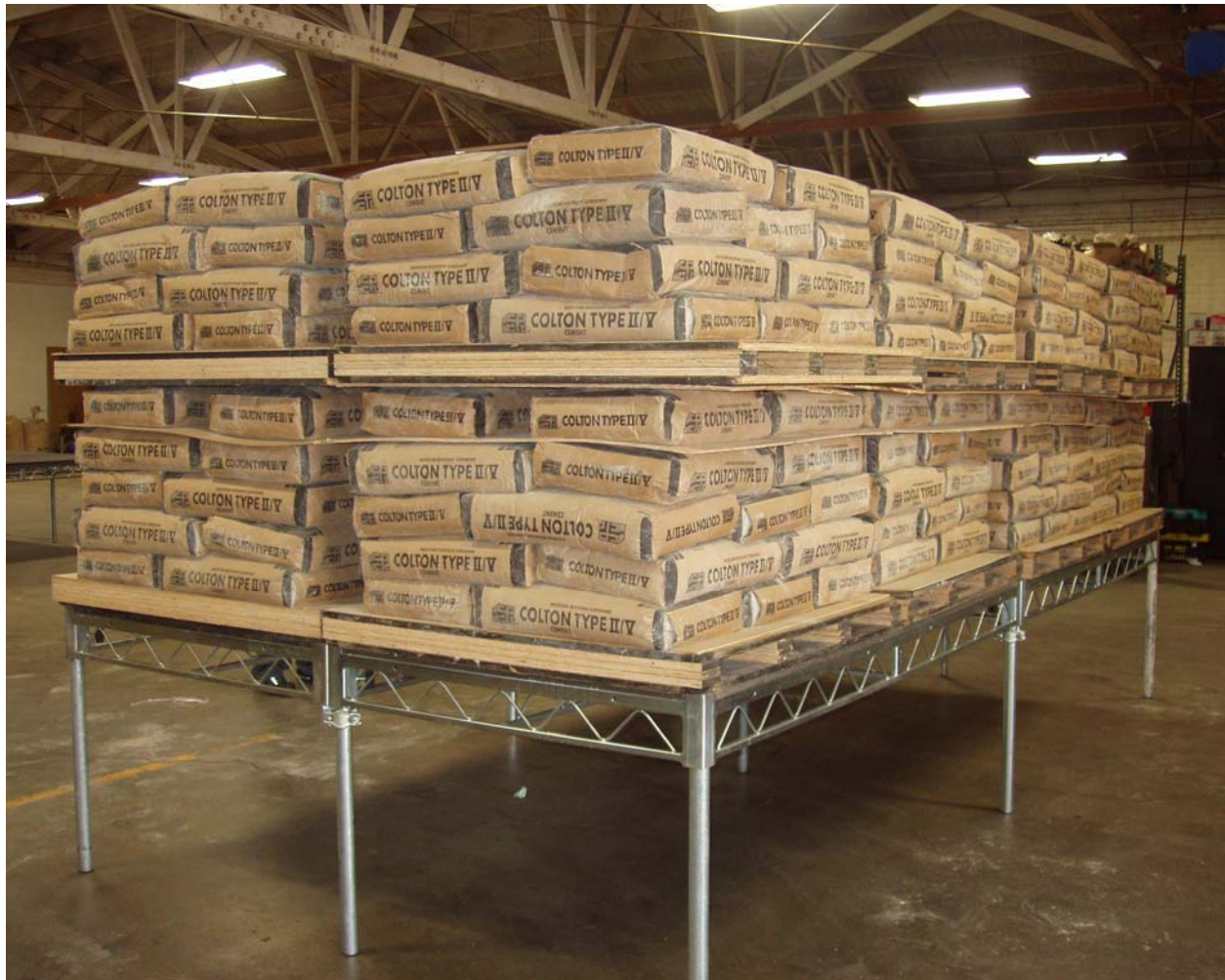
Figure 3-2 Load Step 2, 1 st Platform loaded to 271.0 lbs/ft 2
