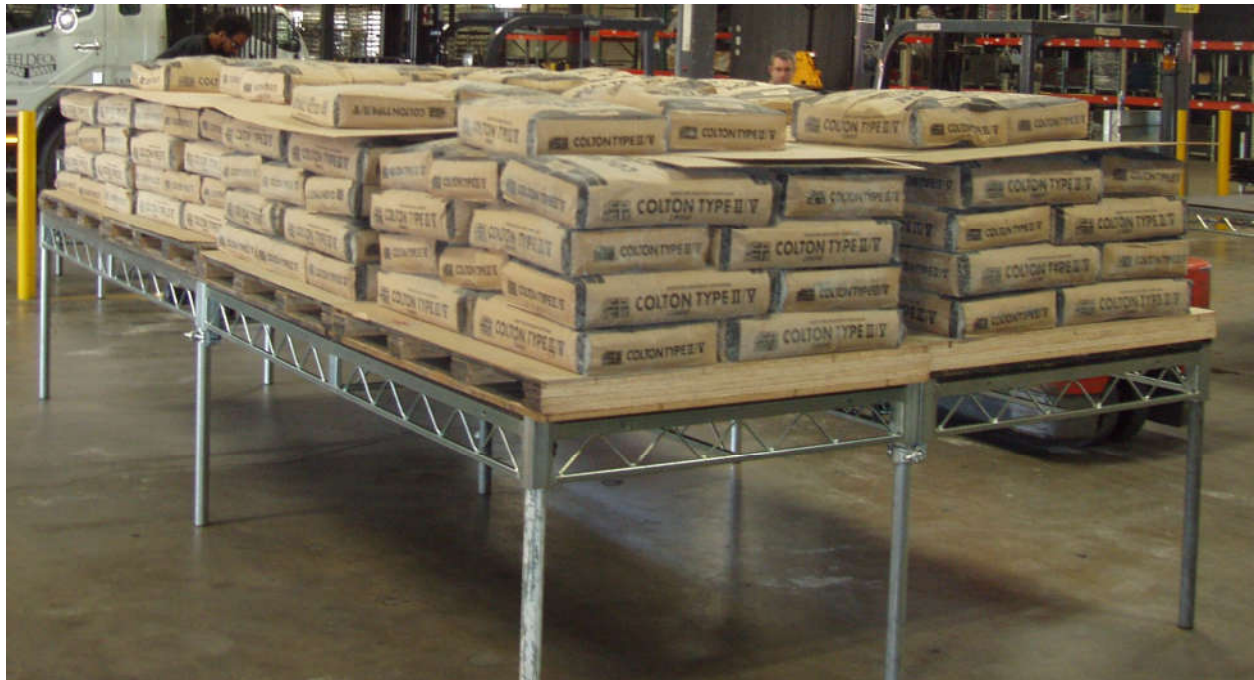
Figure 3-1 Load Step 1, 1 st Platform loaded to 135.5 lbs/ft 2
