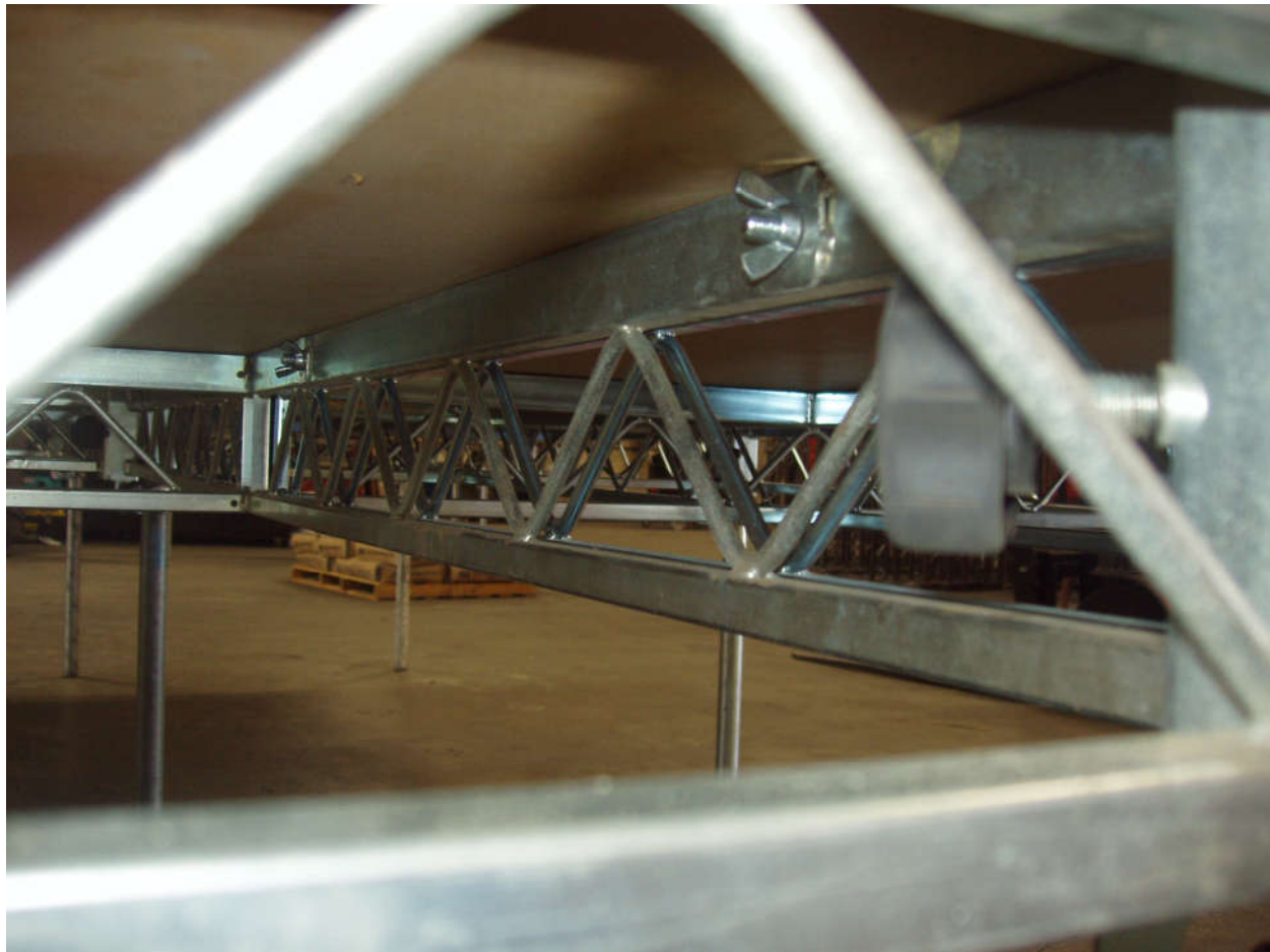
Figure 3-4 Load Step 2, 1 st Platform loaded to 271.0 lbs/ft 2 , Inboard long beams
