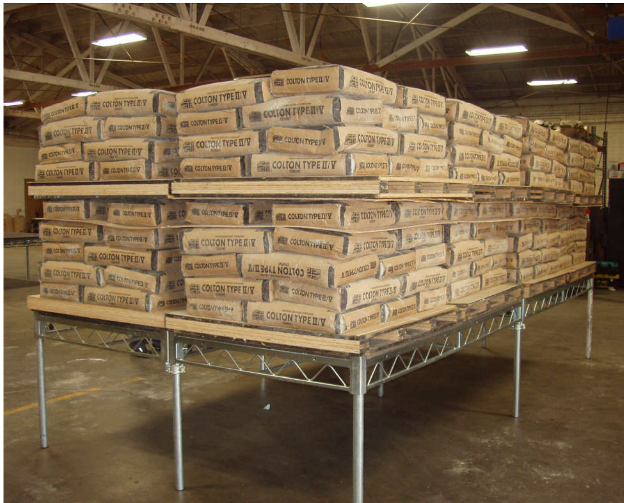
Figure 3-2 Load Step 2, 1 st Platform loaded to 271.0 lbs/ft 2
