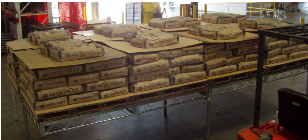
Figure 2-6 First Platform loaded to 135.5 lbs/ft 2
