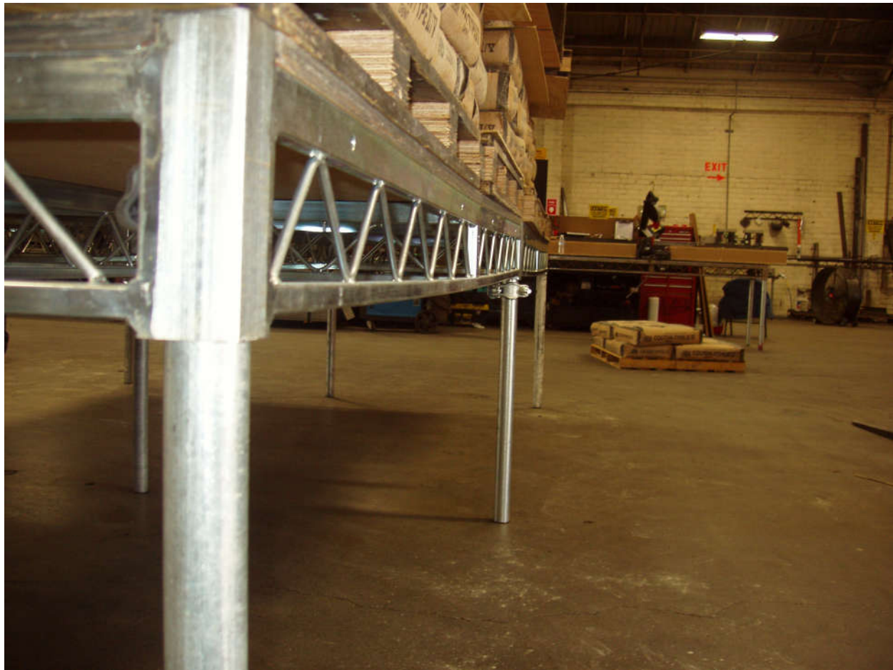
Figure 3-3 Load Step 2, 1 st Platform loaded to 271.0 lbs/ft 2 , Sag of long side beams
