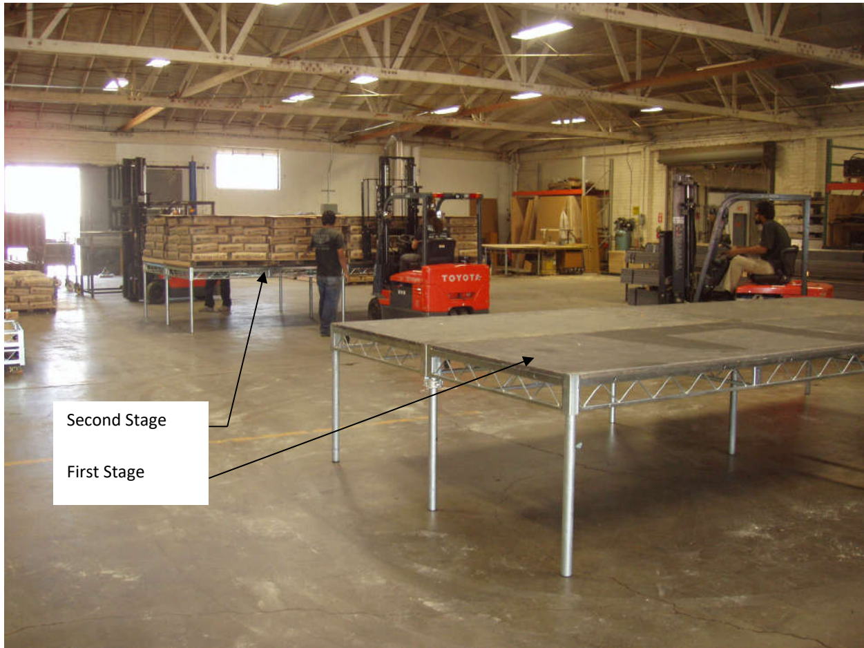
Figure 3-7 Load Step 4, 2 nd Platform loaded to 147.25 lbs/ft 2
