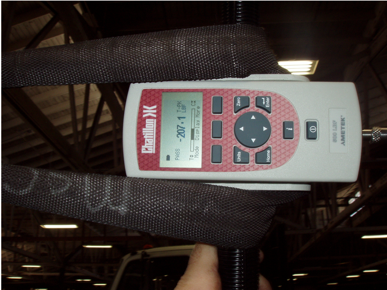
Figure 3-2 Outboard Test #1 loaded to 207.1 lbs
