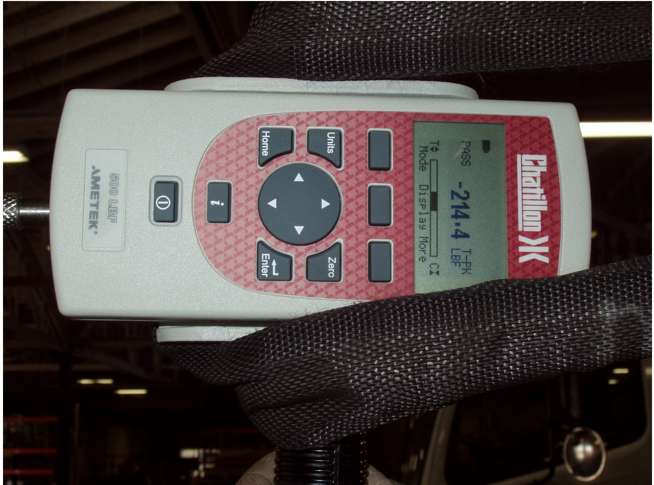
Figure 3-4 Inboard Test #2 loaded to 214.4 lbs
