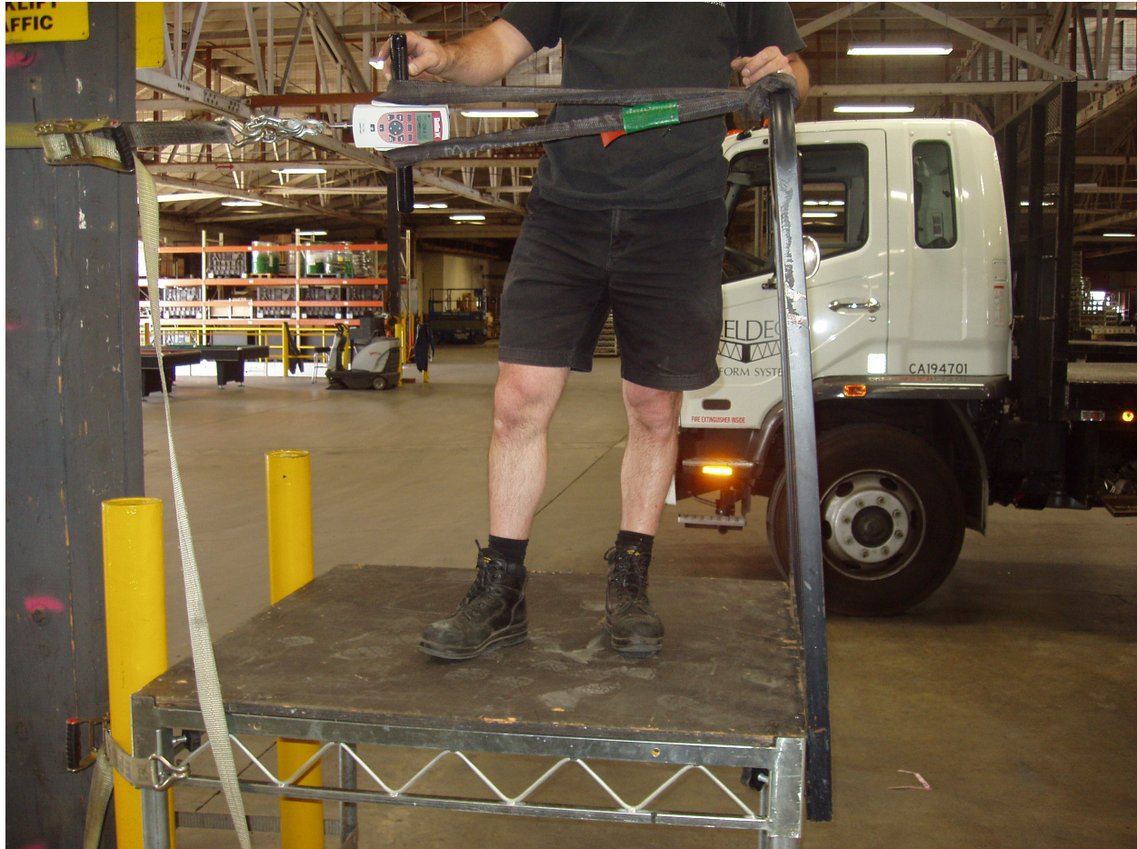
Figure 3-3 Elastic Deflection, Inboard Test #2 loaded to 214.4 lbs
