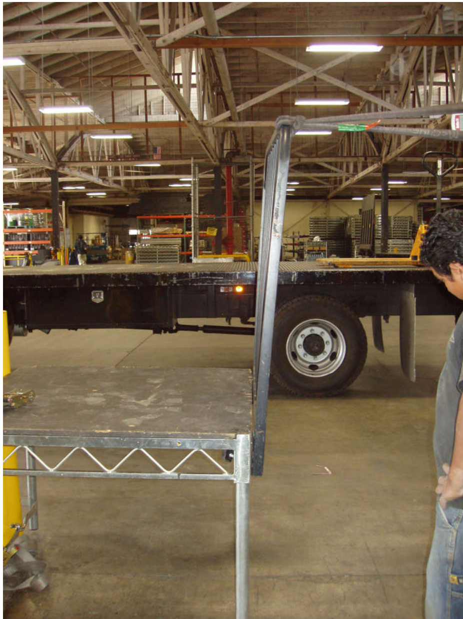
Figure 3-6 Elastic Deflection, Outboard Test #3 loaded to 382.1 lbs
