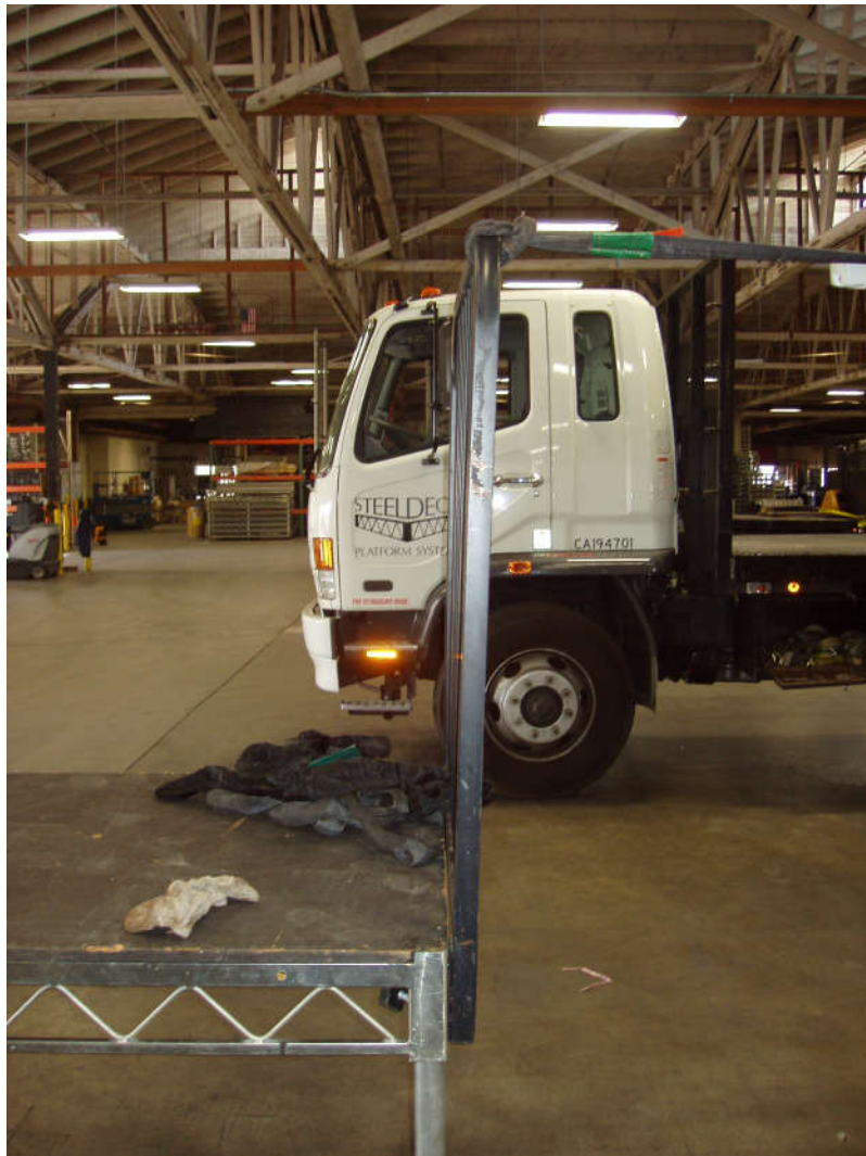
Figure 3-1 Elastic Deflection, Outboard Test #1 loaded to 207.1 lbs
