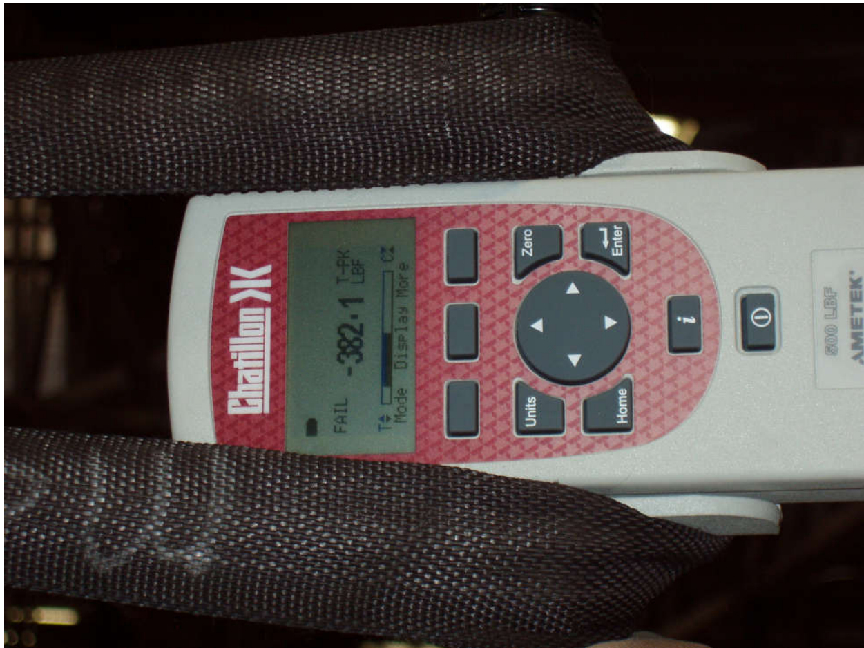
Figure 3-7 Outboard Test #3 loaded to 382.1 lbs
