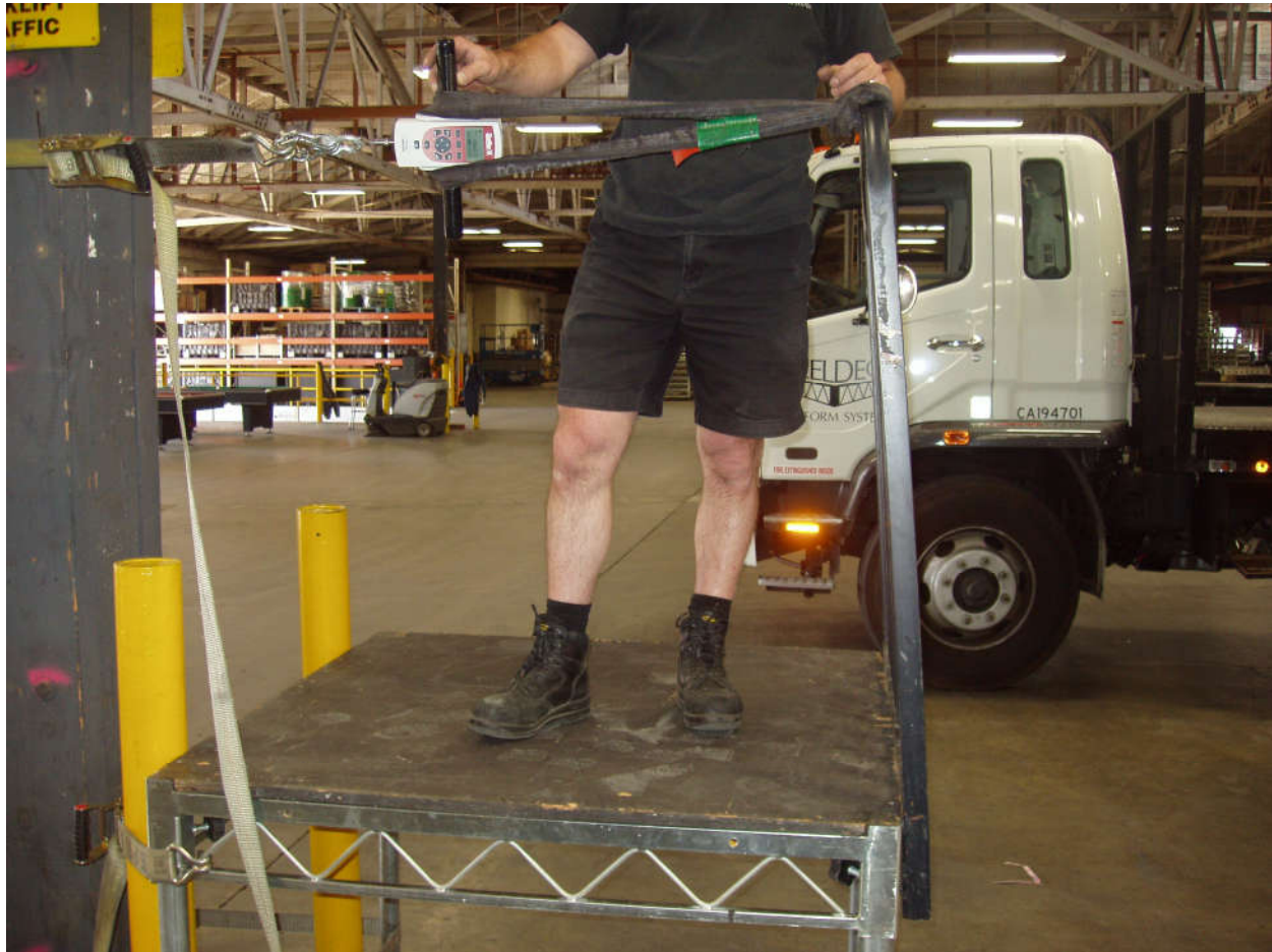
Figure 3-3 Elastic Deflection, Inboard Test #2 loaded to 214.4 lbs
