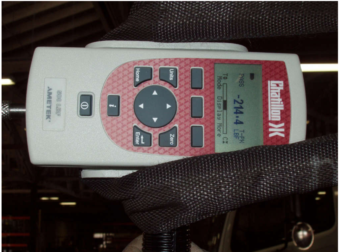
Figure 3-4 Inboard Test #2 loaded to 214.4 lbs
