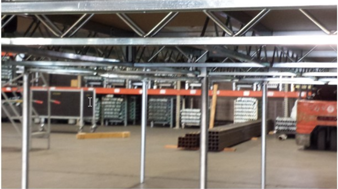
Figure 3-6 Load Step 4, Platform loaded to 202.76 lbs/ft 2
