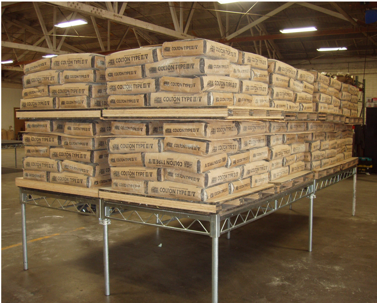
Figure 1-6 3 Ft High Platform loaded to 271.0 lbs/ft 2
