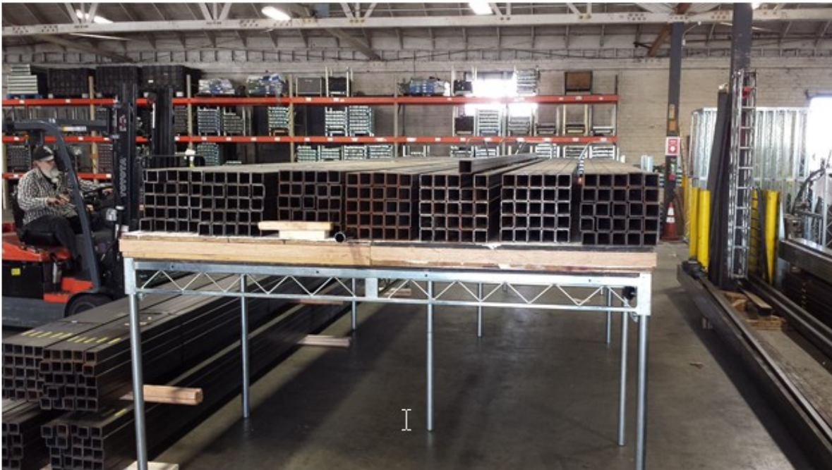
Figure 3-1 Load Step 2, Platform loaded to 102.9 lbs/ft 2
