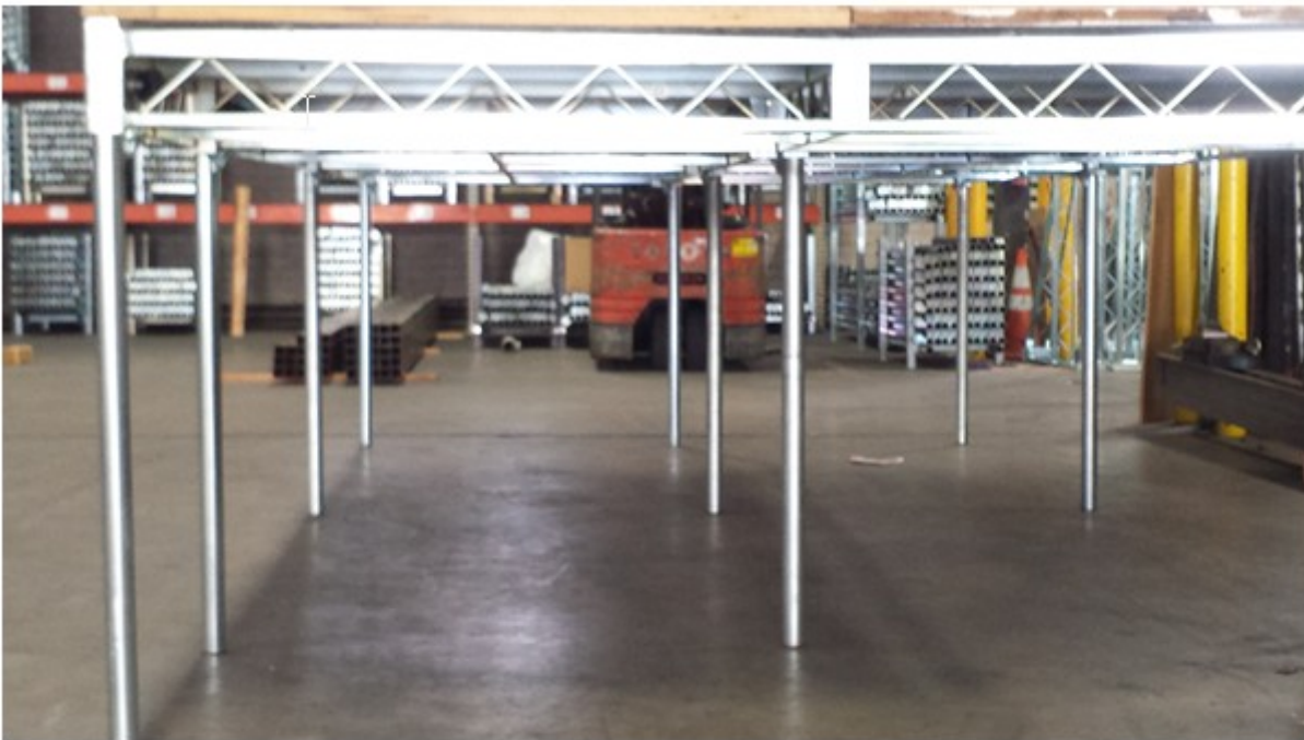
Figure 3-5 Load Step 4, Platform loaded to 202.76 lbs/ft 2
