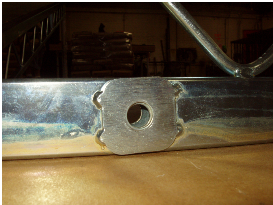
Figure 3-8 No distress of critical deck-to-deck bearing surfaces
