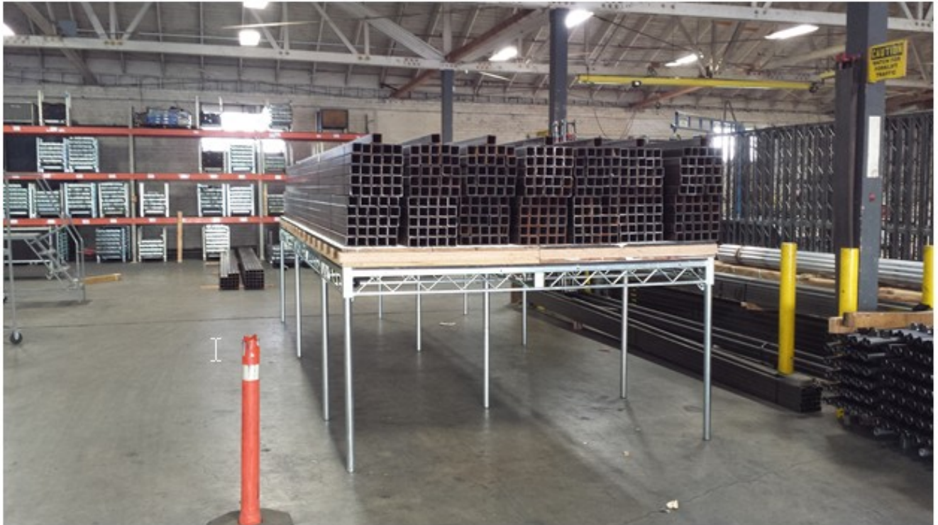
Figure 3-3 Load Step 4, Platform loaded to 202.76 lbs/ft 2
