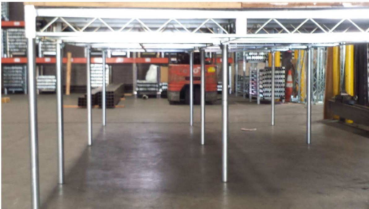
Figure 3-5 Load Step 4, Platform loaded to 202.76 lbs/ft 2
