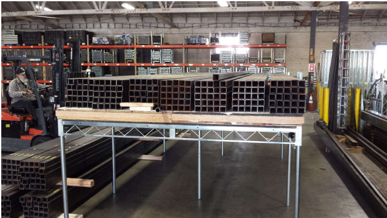
Figure 3-1 Load Step 2, Platform loaded to 102.9 lbs/ft 2
