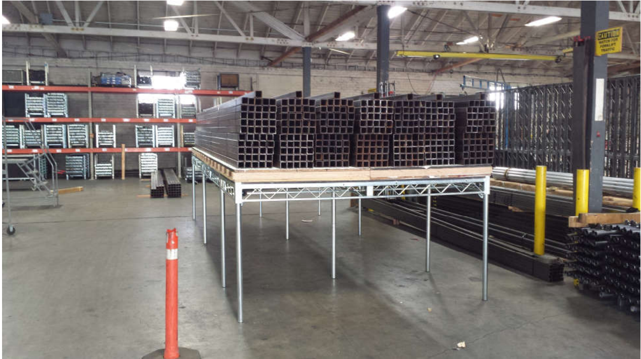
Figure 3-3 Load Step 4, Platform loaded to 202.76 lbs/ft 2
