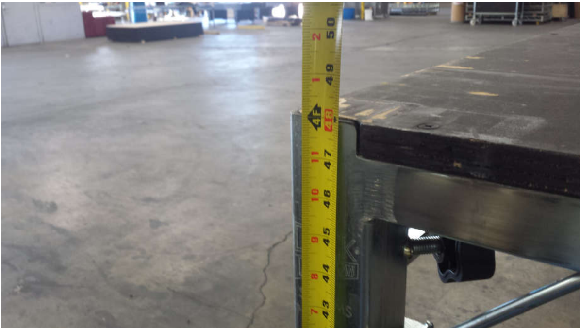
Figure 2-2 Test Platform, 4 ft high measured
