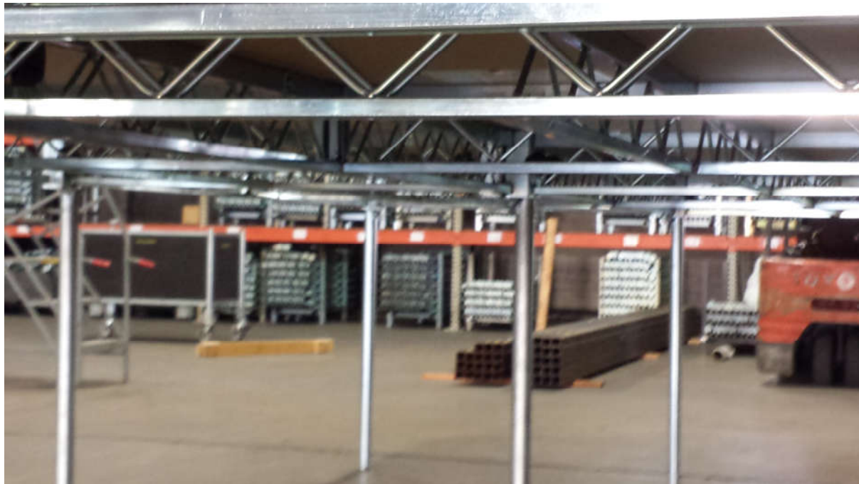
Figure 3-6 Load Step 4, Platform loaded to 202.76 lbs/ft 2
