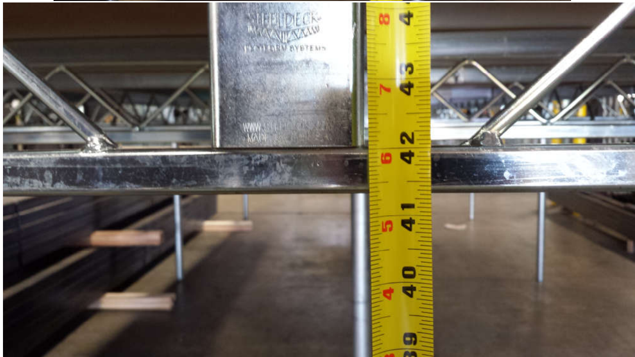
Figure 3-2 Load Step 3, S/N 22065 Deck max deflection, typical all decks @ 102.9 lbs/ft 2
