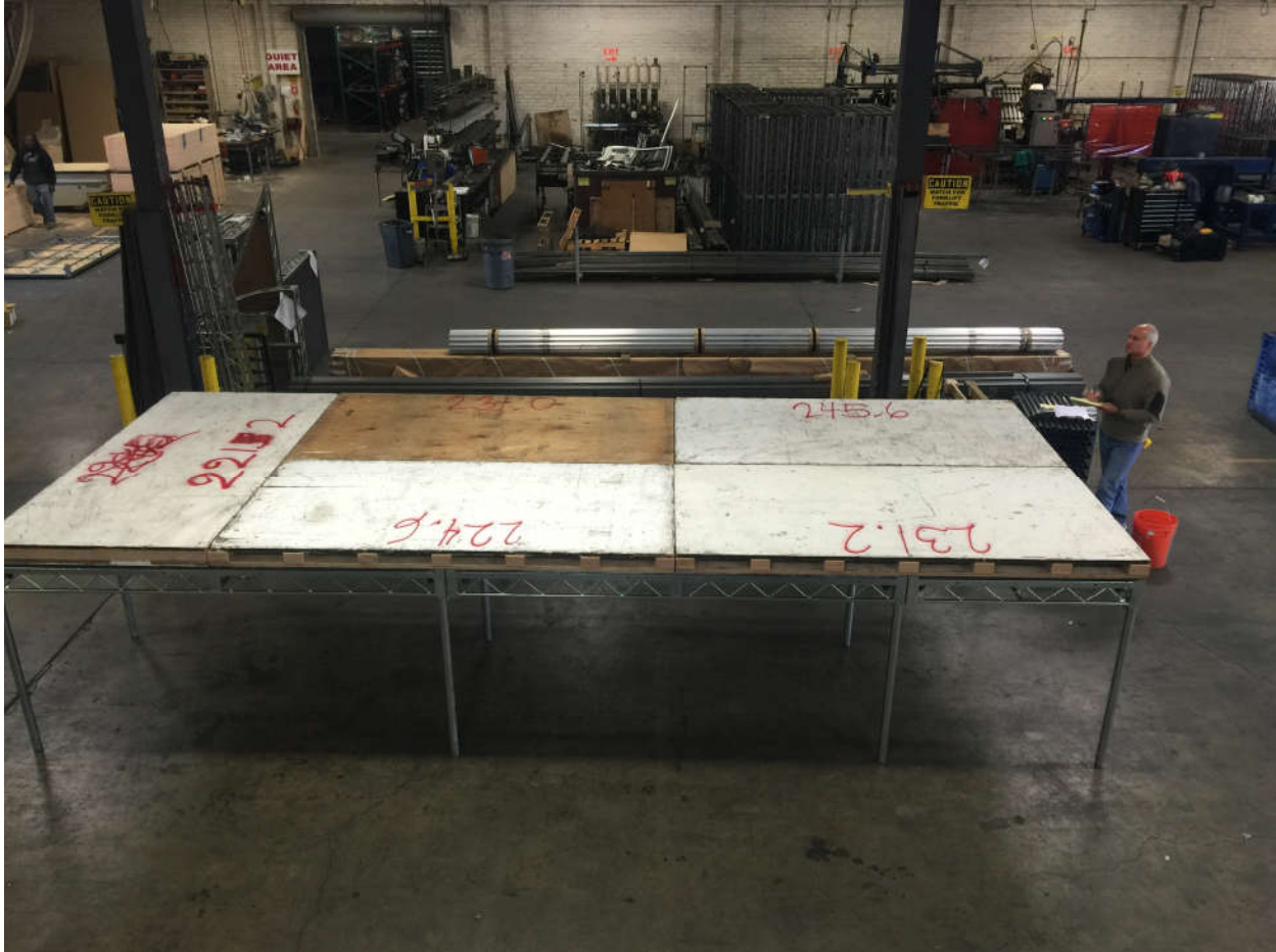
Figure 2-9 4 ft. tall 8x20 ft. Platform with \geq 221 lb wooden pallets in place, overlapping deck seams
