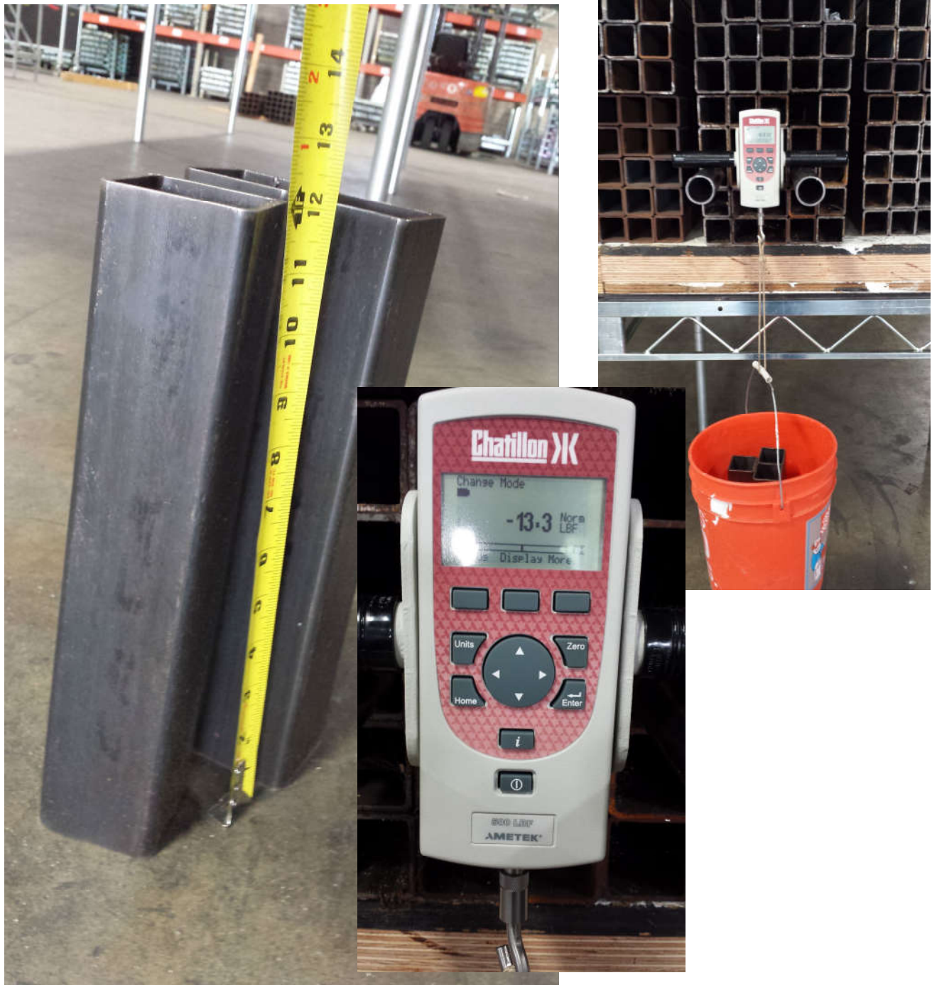
Figure 2-6 Weight of three feet of unit tube stock, 13.3 lbs → 4.433 lbs/ft
