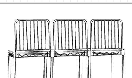
Guardrails are modular and do not interconnect. Units comprise the guardrail, two backplates and two hand knobs. Guardrails are fixed as follows:
