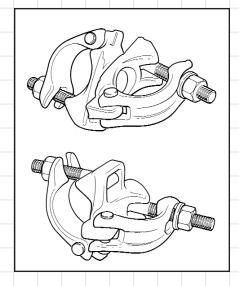
Stages built over four feet high must be cross-braced with horizontal and diagonal lengths of 1½ Schedule 40 pipe for stability and safe use. Bracing must be secured with standard fixed (two way) and swivel clips. All bracing components are available from Steeldeck, Inc.
