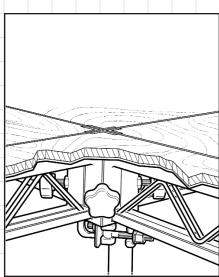
Couplers allow Steeldeck® platforms to be cross-braced when built above 4 feet high or on screwjacks or casters.
